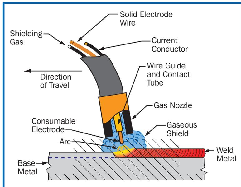
FIGURE 2. MIG welding process.
