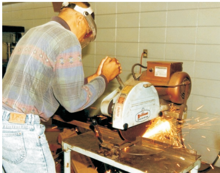
FIGURE 3. Cutting metal with a cutoff saw.
